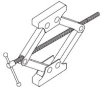
The device is modelled by a rhombus, with each side 25cm. The horizontal length is x cm, and the vertical height is h cm as shown.
